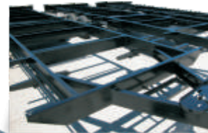
Additional Welds Create Camber in the Chassis for Greater Load Carrying Capacity
