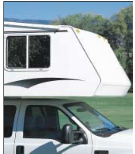
An aerodynamic molded fiberglass front cap reduces wind resistance and provides spacious headroom in the bedroom.
