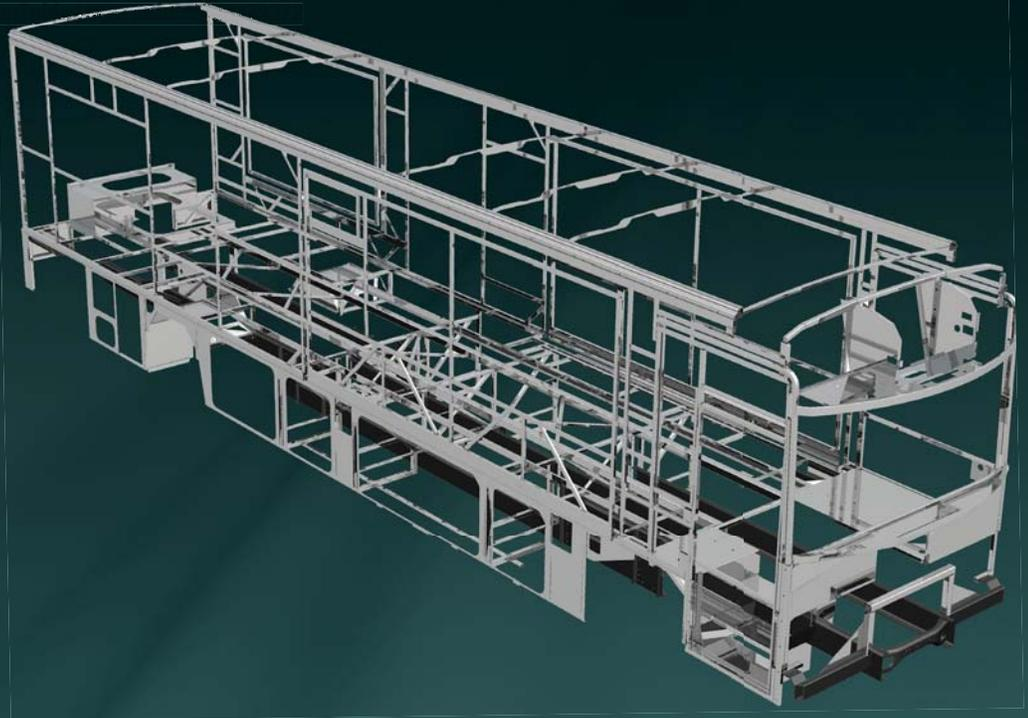
**SuperStructure®** Legendary strength and durability are the results of SuperStructure construction that goes into every Itasca motor home. It's the combination of quality, proprietary components and careful attention to detail that makes Itasca motor homes the cream of the crop.
