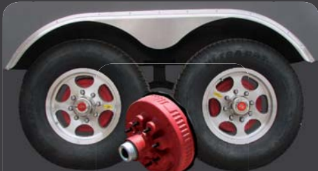
16" Load Range "E" Radial Tires with 6000 Lbs. Axles
